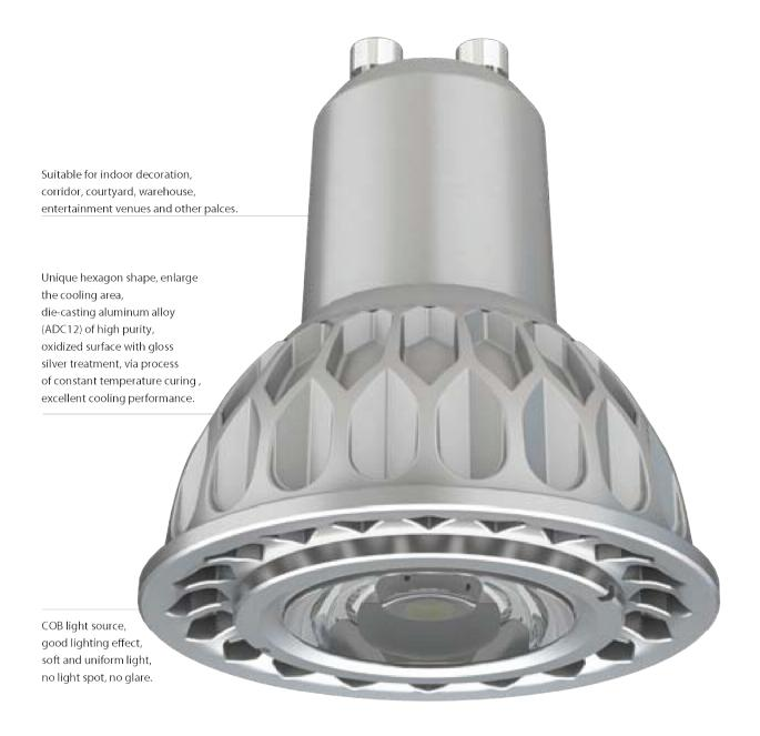
High bright CREE COB LED, CRI >80, built-in isolated driver, high light efficiency, lumen of neutral white >90LM/W.
